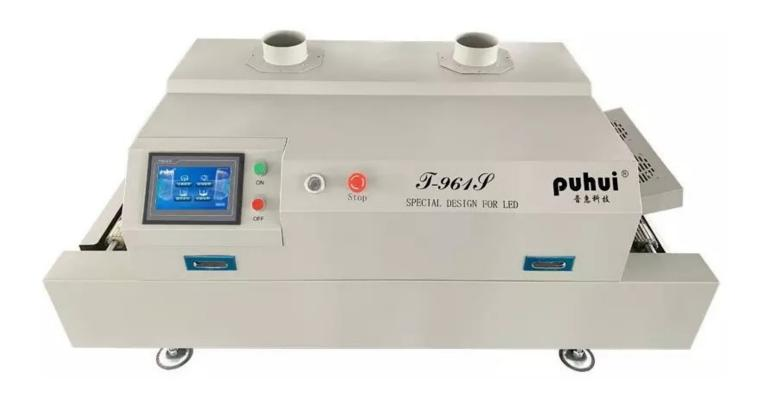
Smart touch screen PCB welding machine T961S six heating zones SMT infrared conveyor **Reflow Oven**
