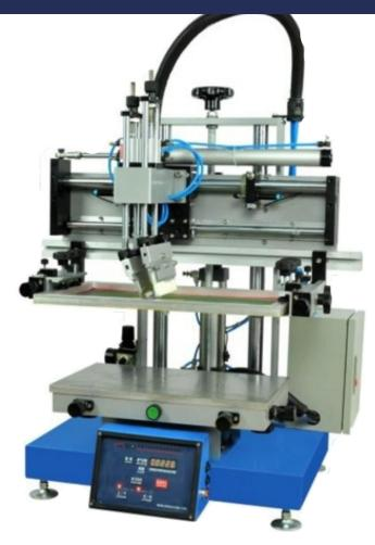
SP-2535 is a semi automatic solder paste printer. This machine is similar to the full automatic printing machine, the scraper can freely move up and down and automatically adjust the level with stencil. But the alignment and loading of PCBs has to be done by manually.
